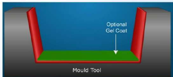
Basic Process of Hand Lay-up
